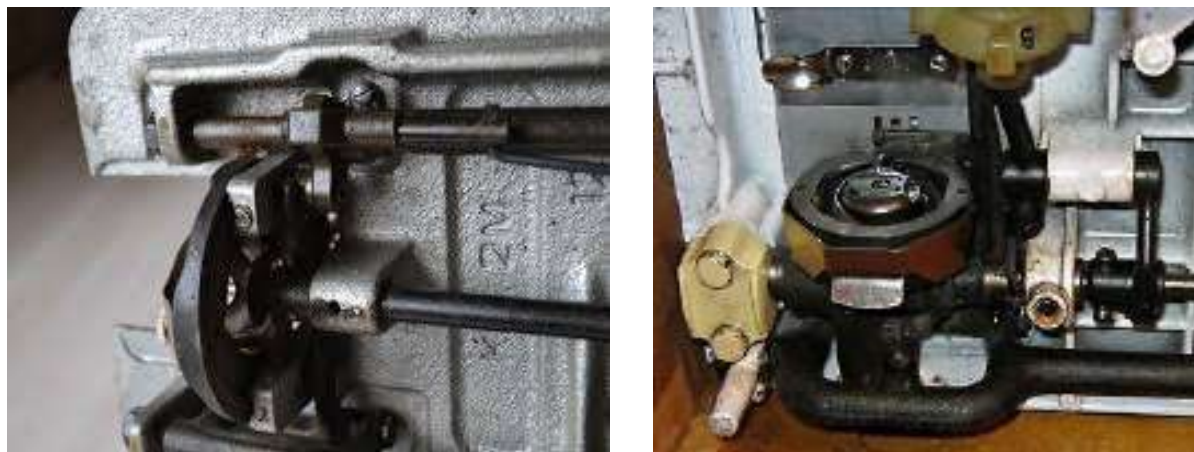
Figure 5. The process of installing a shuttle automatic filling device
