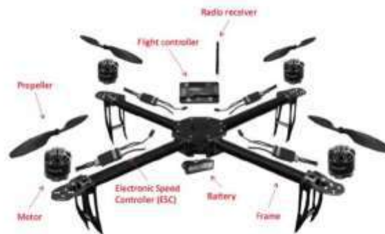
Figure 1. Architecture of a quadcopter
